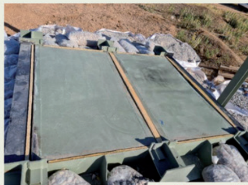
Fig. 6 Permanent deflections after the explosion
